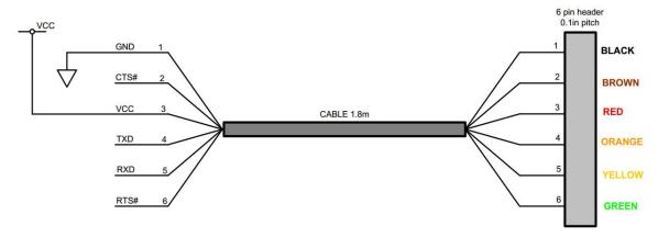
Because, of the current limit of the FTDI chip, another cable should be used for supplying the device. Recommended solution:
