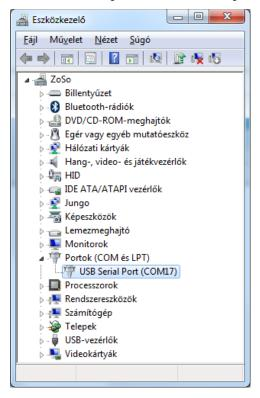
As you can see, in this case we are using a USB-serial converter that provides us with a virtual serial port named COM17. Please make sure that the serial port is not opened by any other program (eg. terminal emulator). Now we may proceed to the actual flashing of the device.
